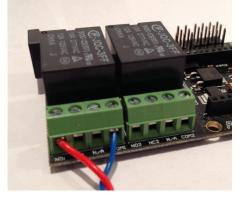
Connect one of the DFRobot Xboard relays to your existing garage door opener wall button. This will require the installation of 2 low voltage wires going from one of the terminal blocks labelled COMx and NOx, to your existing garage door wall mount button station (the 'x' in COMx and NOx is a value between 1 and 2).
